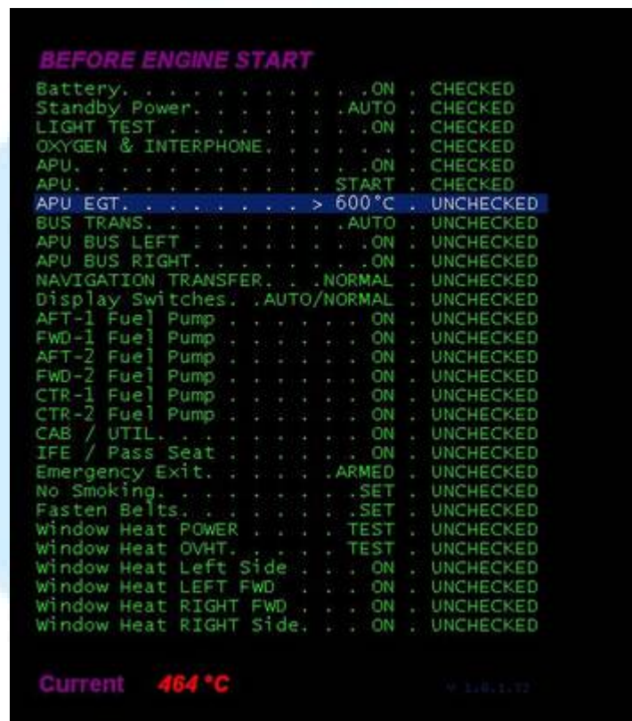
The system in Autocheck mode waits for minimum APU EGT to set the CHECKED status
